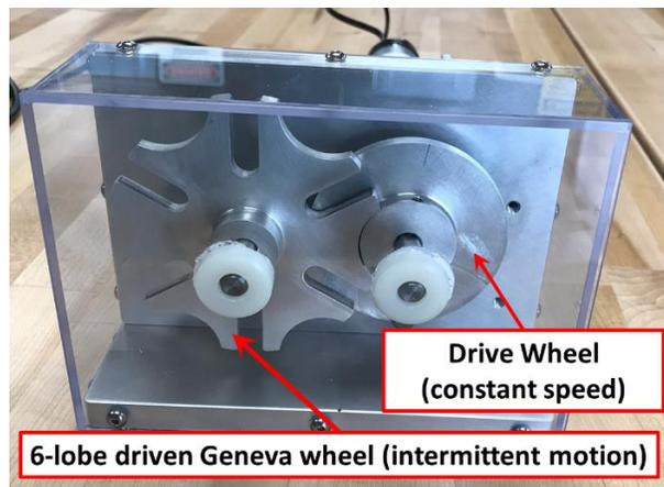
**Figure 3.** Front view of the completed Geneva mechanism. Drive wheel at right is connected to the electric motor drive mounted at the back and rotates at a constant rate. The six-lobe driven wheel at left moves intermittently.
