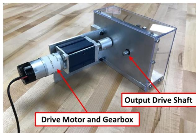
**Figure 4.** Rear view of the completed Geneva mechanism showing mounting of electric motor drive and stub shaft that can be used to harness the intermittent motion of the Geneva wheel.
