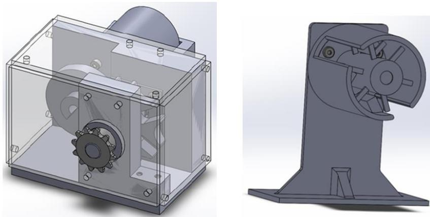
**Figure 2.** Left: CAD model of assembled Geneva device. Case of driver motor is shown at rear. Gear wheel on front of case is provided to drive application requiring timed intermittent application such as loader mechanism for walking beam conveyer. Right: CAD model of loader mechanism to load parts on walking beam at specified feed rate.
