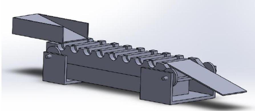
**Figure 1.** CAD model of assembled walking beam conveyor component. Parts are to be to the chute at left by the feeder mechanism operated by the Geneva mechanism. The outer rack is stationary while the inner rack is moved by an eccentric drive mechanism. This motion moves the parts intermittently to the right.
