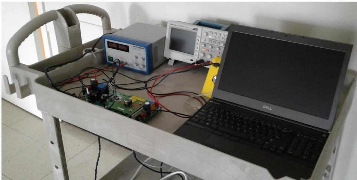
Figure 1. Power electronics mobile lab bench setup
