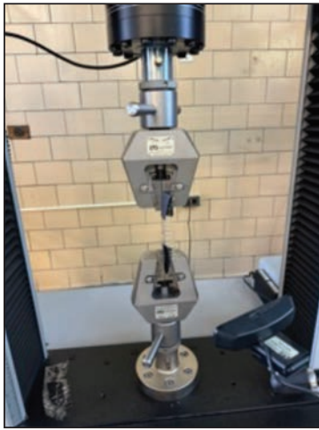
Figure 3. Tensile strength test of plastic sample.
