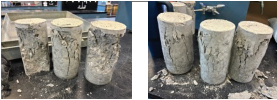
Figure 6. Fractured specimens after 28-day compression test (a) control concrete (b) 20% plastic added concrete.
